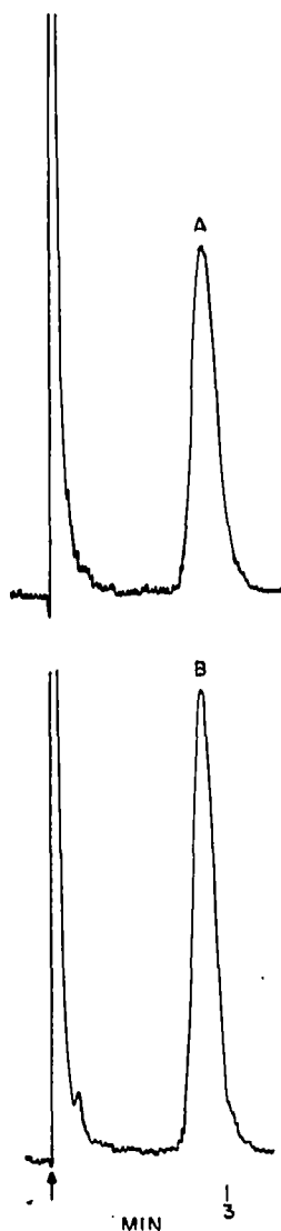
Fig. 1. Gas chromatogram resulting from analysis of the diheptafluorobutyramide of p,p '-diaminodiphenylsulfone (B) and the product resulting from treatment of p -ureido- p '-aminodiphenylsulfone with heptafluorobutyric anhydride (A). Column conditions: 1 ft. \times 3 mm I.D. spiral glass column; SE-30-CHDMA two-component 3% stationary phase (2.5:0.5) on 80-100 mesh acid-washed and silanized Gas-Chrom P; 240°; 50 ml/min argon. Argon ionization detector: 8 V d.c.; Glowall instrument.
